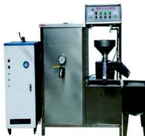
TG-100 Soya Milk Making Machine (Required Boiler additional)
